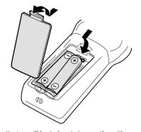
The batteries will last about six months with normal use. If the functions of the remote control become erratic, replace the batteries.
